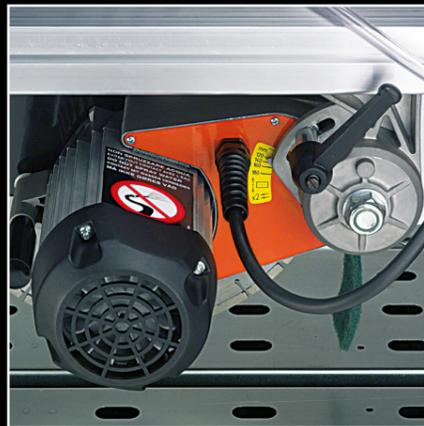
A graduated scale measures the adjustment of the cutting depth by means the locking of the tilting of the engine group.
